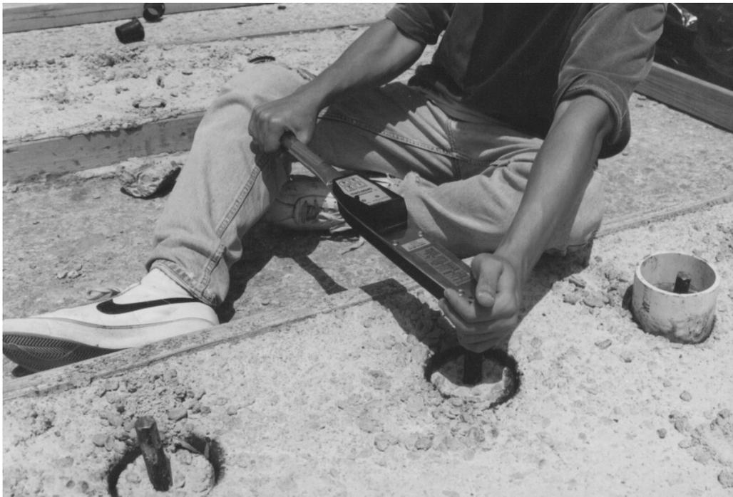
Figure 9. Torsional shear testing in operation.
