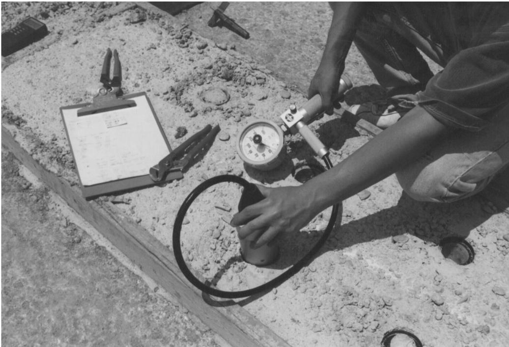
*Figure 11. Break-off testing in operation.*
