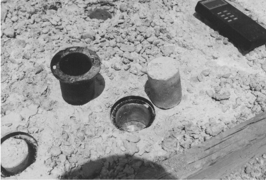
*Figure 10. Break-off test sleeve and sample.*
