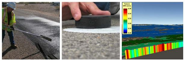
Figure 3 – Constructing undesired texture (a), measuring with sand patch (b), managing pavement texture (c)
