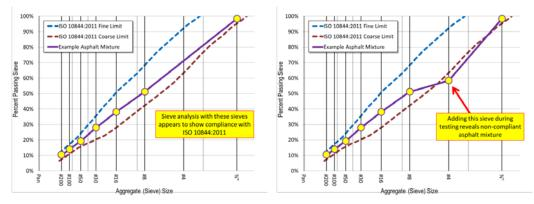
Figure 5 – ISO-specified sieving curve limits, but with discrete sieve testing can show pass (a) or fail (b)
