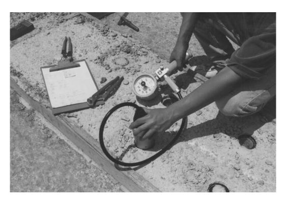
Figure 11. Break-off testing in operation.
