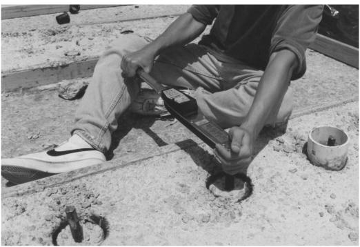
Figure 9. Torsional shear testing in operation.
