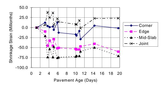
Figure 116. Shrinkage strain at station 701+50.
