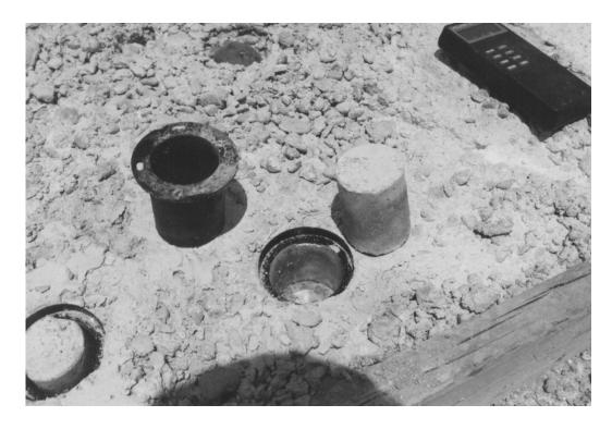
Figure 10. Break-off test sleeve and sample.
