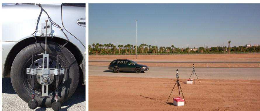
Figure 4. Locations of microphones for measuring tire-pavement noise. (Left: measuring at the source using the OBSI method; right: microphones for wayside measurements)
